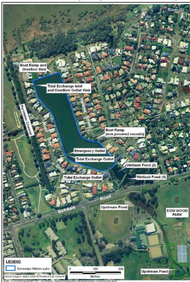
Figure 1 – Sovereign Waters Main Hydrodynamic Components
