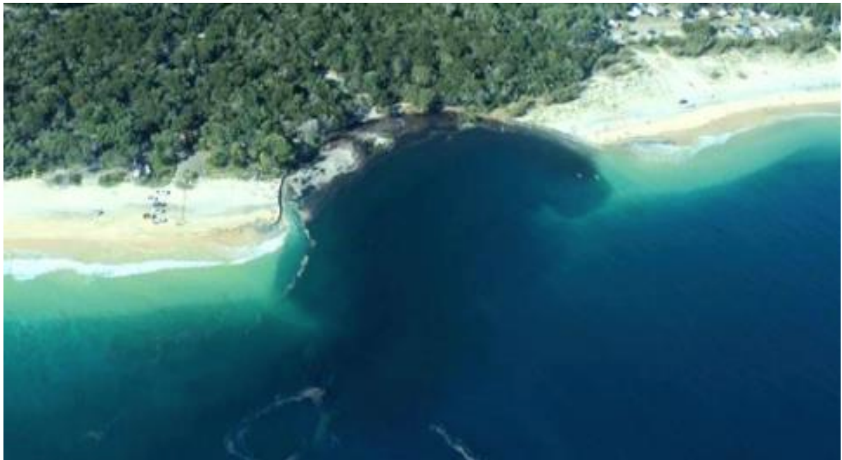
Figure 2. This image shows the amphitheatre shaped crater left after a large RBF event at Inskip Point, Queensland which took place at night on 26 th September 2015. This event retrogressed into a camping area behind the beach and undermined a car and caravan. Many similar events have occurred on this beach.
