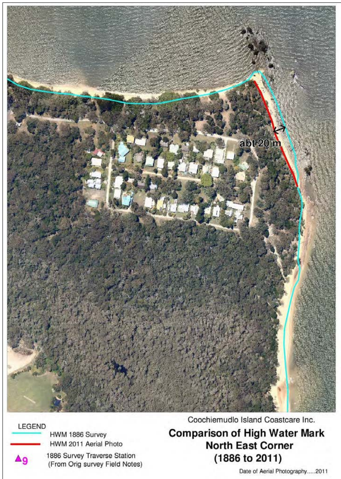
Figure 3-4 Comparison of the North East Corner High Water Mark (Provided by Coochiemudlo Island Coastcare and courtesy of Mr Keith Slack)
