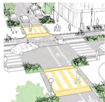
Figure 23: Raised pedestrian crossings at an intersection
